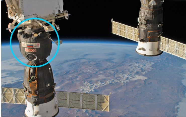
Space station astronauts patched a small hole in the upper orbital module of the Soyuz MS-09 spacecraft (left) on Aug. 30, 2018. Russian space officials have said that hole was likely caused by a drill here on Earth; investigators are currently trying to figure out exactly what happened.
